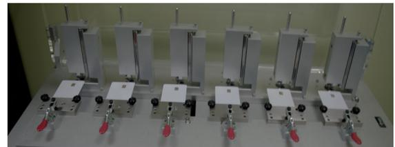
Same equipment than BGI058 above but testing 6 cards together and along 2 axes, for 6 and 8 PINS chips or non-standard chip position (RFID chips, sensors, ...).
