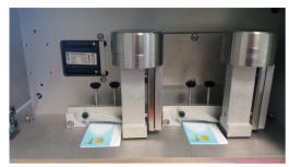
This line of the BGI110 realises the sandpaper rub test. It allows to test 2 cards on 1 test line
