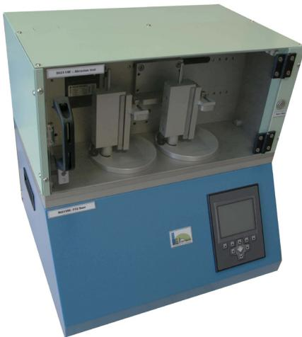
CARD ABRASION «soft eraser rub test» allows to test 2 cards on 1 test line, on the all surface of the card.
