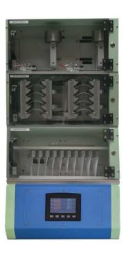
Up to 4 test modules individually managed per PLC
