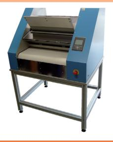
The inlay curvature rectifier has been developed specially for inlay manufacturers. For some productions, inlay leaves manufacturing process not fully flat which causes problem for sheet lamination. This equipment applies a counter force to get the inlay flat.
