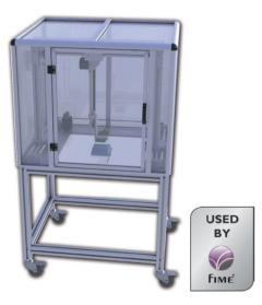
The RFID robot tester has been developed to realize card, passport, reader, smartphone tests in order to check reading distances and compliance of those different credentials.
