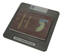
The BGi179 precut tool is used to prepare the passport before the peel strength test is performed on BGI175P.
